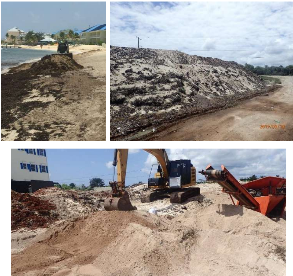
FIGURE 5: SITE VISIT PHOTOS SHOWING THE USE OF HEAVY MACHINERY FOR BEACH CLEANING AND THE RESULTING SAND REMOVAL IMPACTING THE BEACH PROFILE (SOURCE: DOE 2019)
