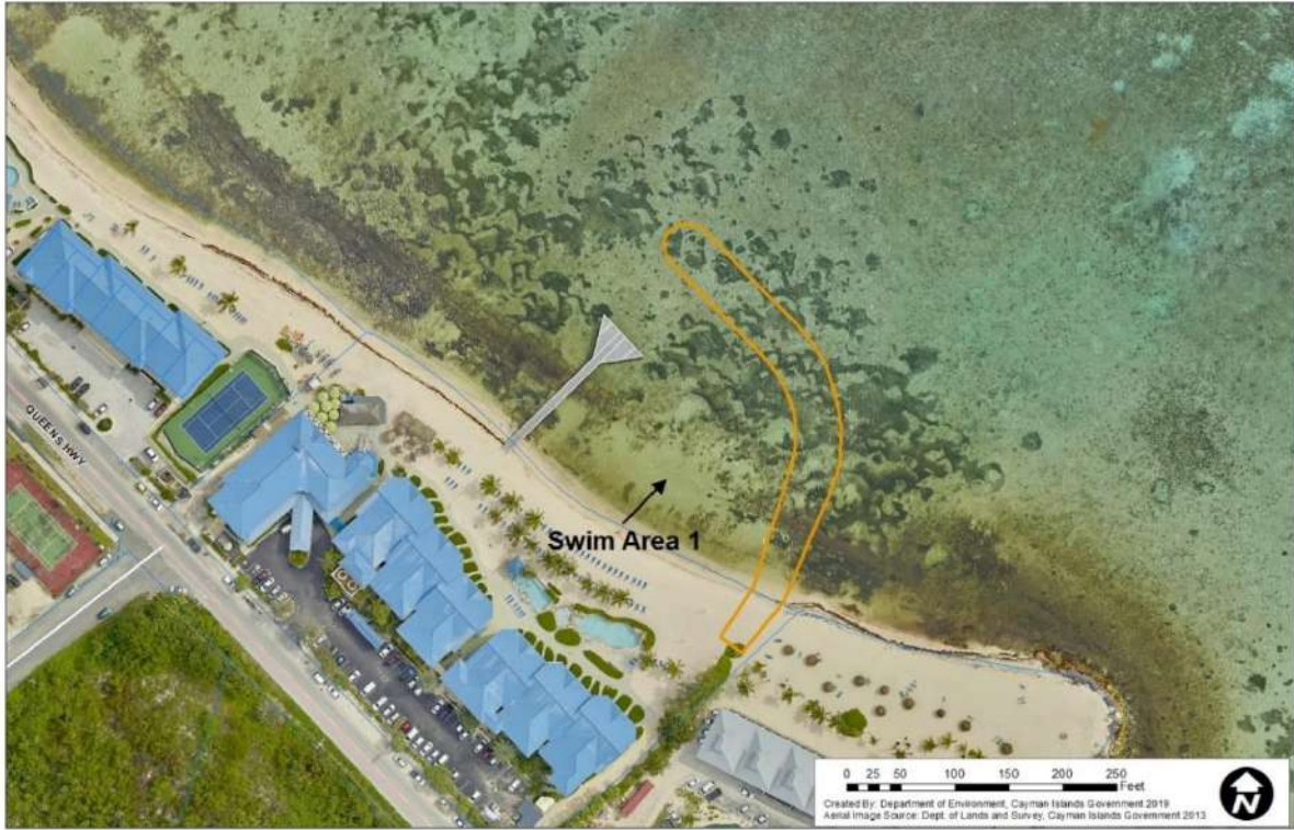
Figure 1. Site Location Plan showing the proposed groyne (outlined in orange) (LIS, 2018 and DOE, 2020).
