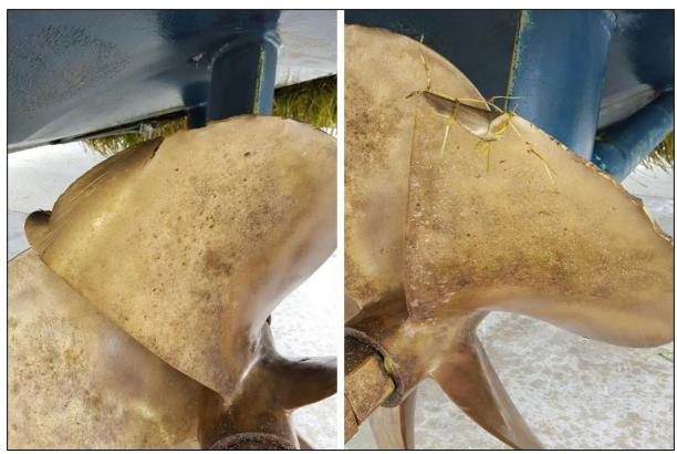
Figure 3 - Shows the damage to the starboard propeller
